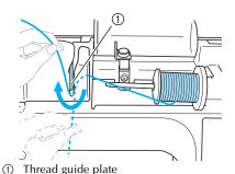
While using your right hand to lightly hold the thread passed under the thread guide plate, pass the thread through the guides in the order shown below.
